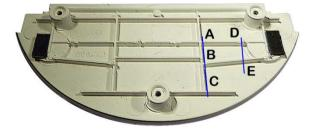
**9.** Modification of the Molding: It is necessary to remove three plastic ribs to accommodate the electronics module located on the underside of the BC7A. It is recommended that you refer to the YouTube instruction video referenced at the top of
